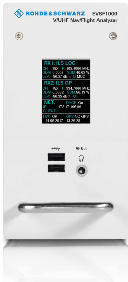
Fig. 3: Since their inner workings are largely identical, comparable measurements are no problem with the R&S®EVSF1000 (left) and the R&S®EVSG1000 (right). The R&S®EVSG 1000 is built to support ground inspection.
