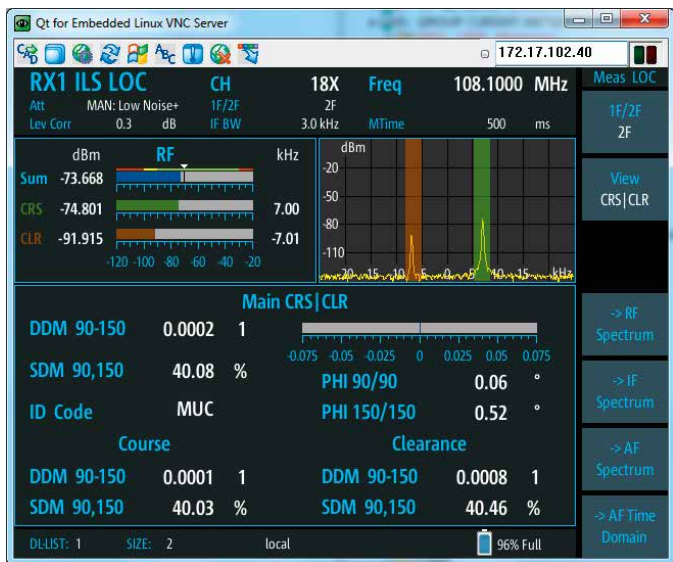
Fig. 4: 2F ILS measurement with IF display of the two carriers (course and clearance), the filter bandwidth settings, the individual measured values (course, clearance) and the sum evaluation.
