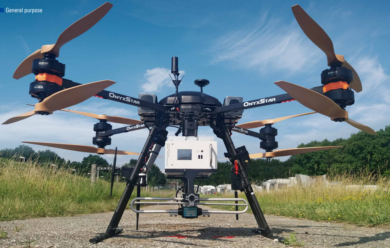
Fig. 1: Measurement flights with drones (here, the R&S®EVSF1000 is installed) are used in ground inspections to reach hard-to-access places (photo: Skyguide).
