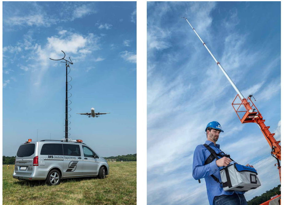
Fig. 2: When performing ground inspections on localizers, certain antenna heights are recommended that are best obtained using a suitably equipped test vehicle. To perform dynamic runway measurements, such a vehicle is needed anyway. For glide slope measurements, the antenna must be positioned even higher.
