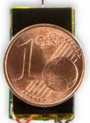
Fig. 3: The ICARUS tag (a virtually series-ready prototype is shown here in actual size) was developed jointly by the Max Planck Institute for Ornithology and I-GOS. It is an autonomously operating multi-sensor device with a radio module (see the overview box on the left for the sensors). The tag communicates with the ISS and with terrestrial base stations.
