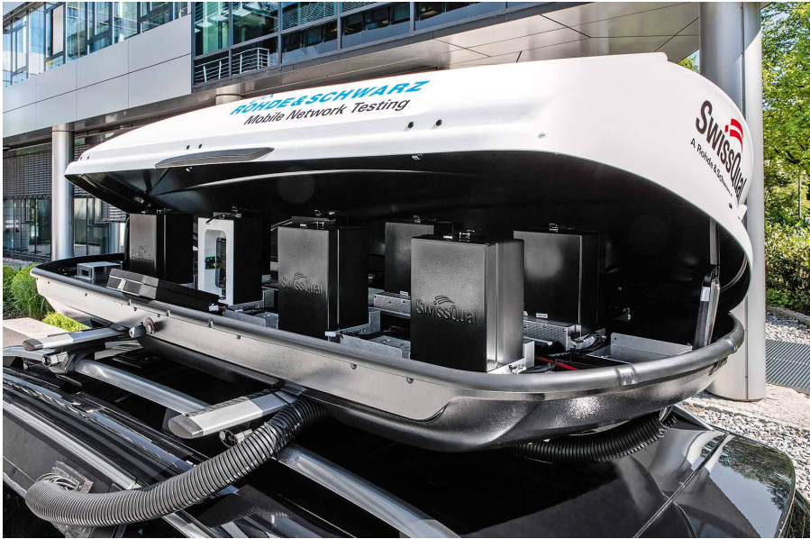
Fig. 6: Vehicle based test campaigns can be used to prepare comprehensive mobile coverage and quality maps. Speech quality measurements are part of the procedure.
