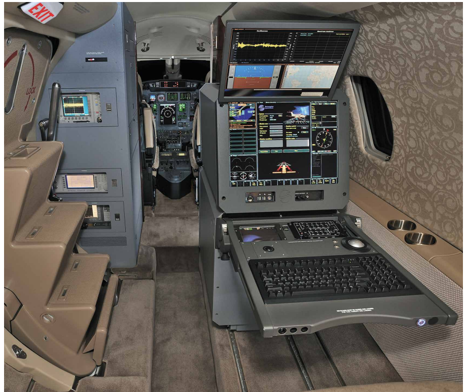
Fig. 7: A typical R&S®EVSF1000 installation in a flight inspection system (photo: Norwegian Special Mission).
