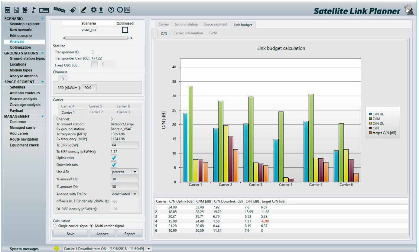
Fig. 3: Calculation of all relevant C/N values after analysis of a multicarrier scenario.
