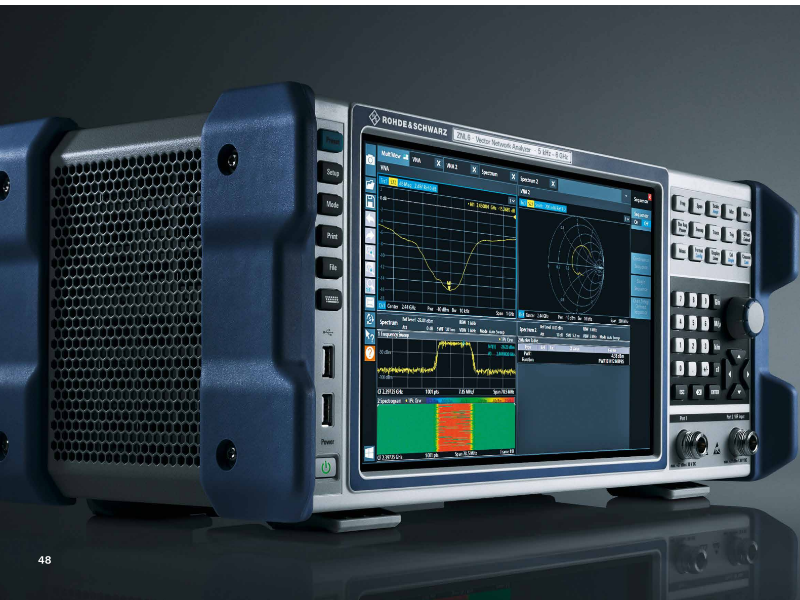
Fig. 1: Not only visually related: The R&S®ZNL vector network analyzer and the R&S®FPL1000 spectrum analyzer are based on the same platform.
